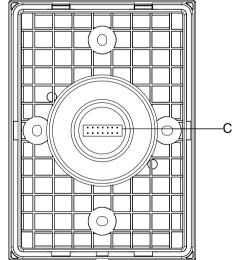
Before mounting the reader onto desired location. Please set the NODE ID (DIP Switch, binary number system). The position of the components varies according to the reader's model. Kindly take note of the components during
